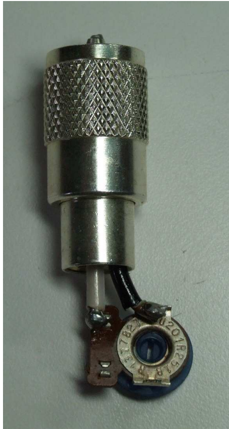
Figure 1 – Variable Resistor Load
