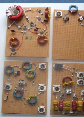
Standard construction using double layer of perfboard, trimmers & silver mica caps, and inductors wound on #2 (or #1) iron cores.
