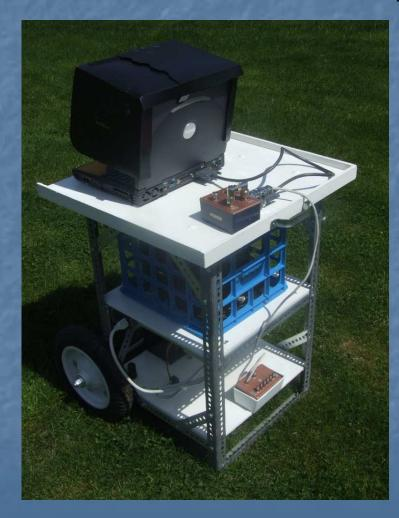
Field Kart Unit 2000 (FKU2000) Laptop w/sun shield Multiplexer Cables/Hardware 12 V Tractor Bat.
